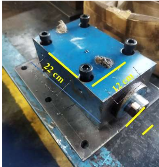
Gambar 1. Shaft Bottom Mold
